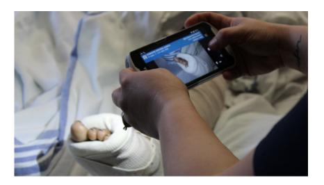
the TC51-HC mobile computer in just one minute, instead of the 10 minutes they used to spend disinfecting an isolation cart, not to mention the individual devices. In fact, the Zebra TC51-HC's are built using Ingress Protection (IP) sealing that allows fast and safe disinfecting because it keeps liquid disinfectants from reaching the electronics.
